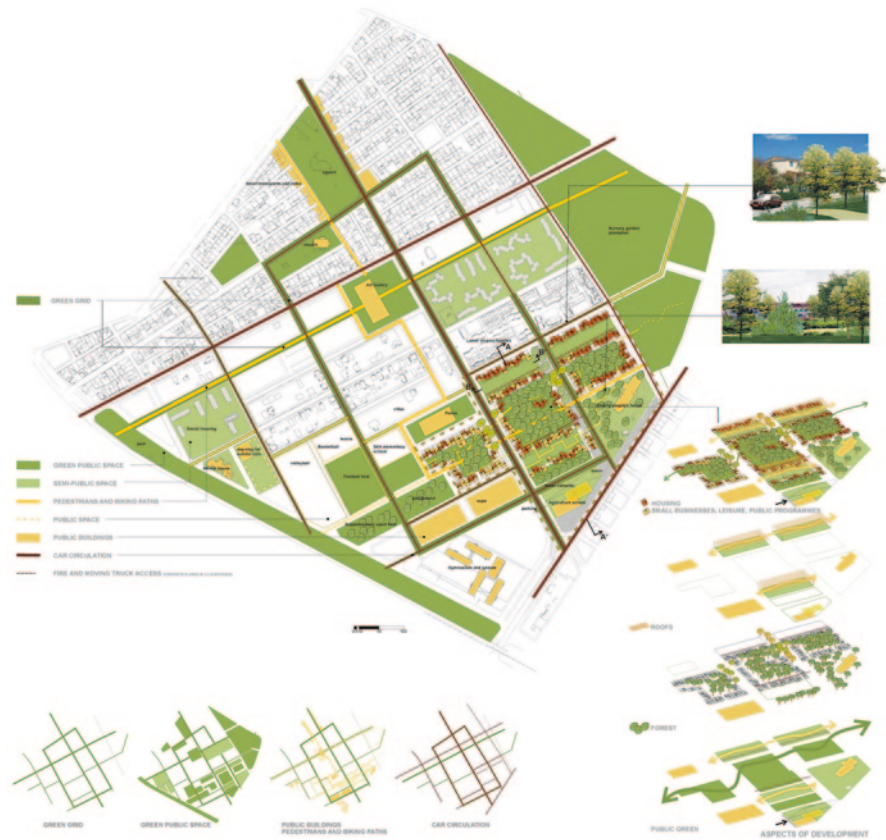
Fig. 8.2 Master plan of the under study area of the old flea market in Neapolis Larissa in Greece with introduction of a bicycle network and a green grid (walking routes)
